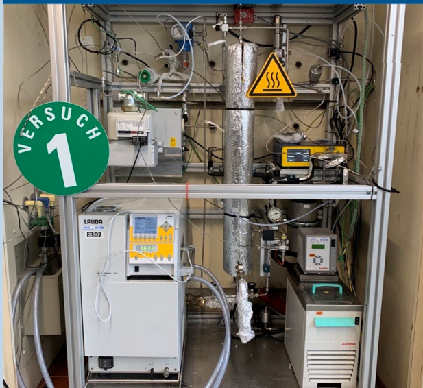
Adsorbent/catalyst testing (@p/T)
