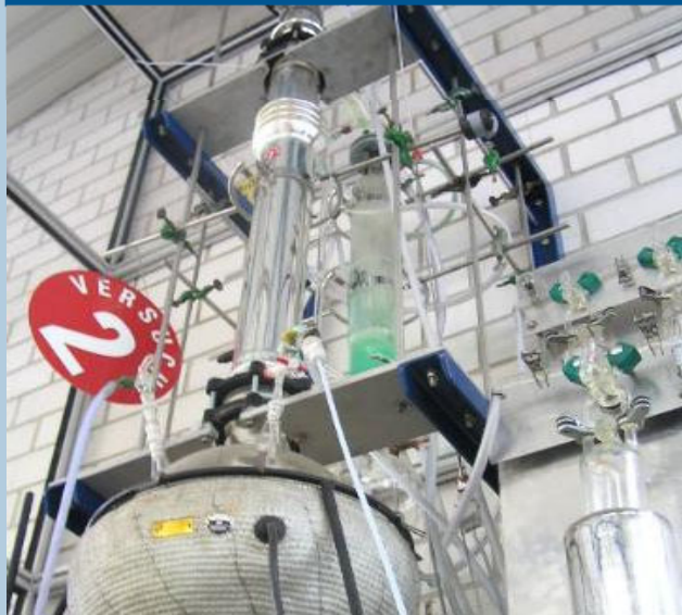
Vacuum Distillation (20 L)
